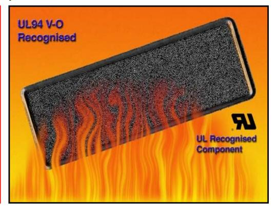
The unique construction of this filter, with strong corrosion resistant wire frame thermoplastically encased and heat bonded to flame retardant media, provides the flexibility to produce the filter in virtually any required size or shape. The post treated, polyurethane, open cell foam media is available in a variety of porosities and thicknesses, all displaying excellent dust holding capabilities when compared to equivalent metal mesh or disposable filters.
