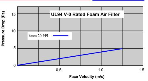
As the filter becomes laden with dust the initial pressure loss will increase. The final recommended resistance is reached when the initial pressure drop has increased by 65 Pascals. The arrestance efficiency of 65% EU2 is based on the filters ability to hold synthetic dust by weight, the test dust particle size ranges from 0-80 microns. The filter efficiency will peak at 1 m/sec, with a reduction likely to be seen when operated above this.
