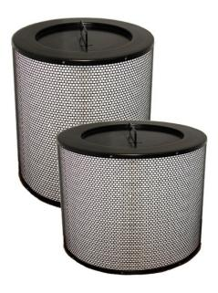
In most HEPA applications it is recommended that a good quality prefilter is installed upstream of the high efficiency filter to alleviate clogging by coarser particles and so extending filter life. Two stage elements, combining pre-filter and high efficiency filter in one unit, offer a convenient integral filter where space is at a premium.
