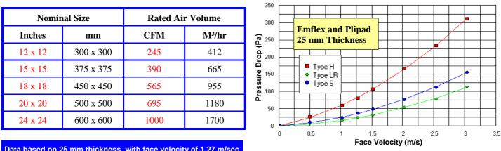
Data based on 25 mm thickness, with face velocity of 1.27 m/sec where efficiencies peak on Emcel Cleanable Panel Filters
